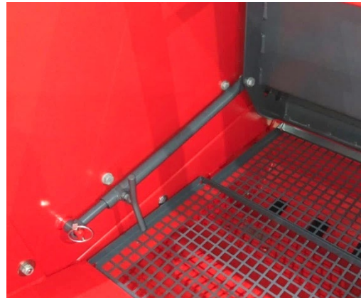
Picture 8. Container dividing wall control rod.
