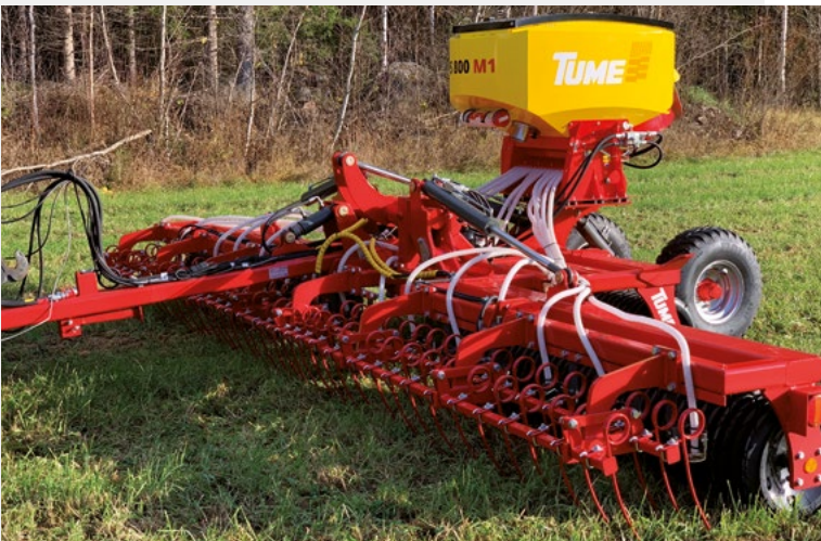
DOUBLE ROW FRONT HARROW. TWO DIFFERENT TINE OPTIONS.
