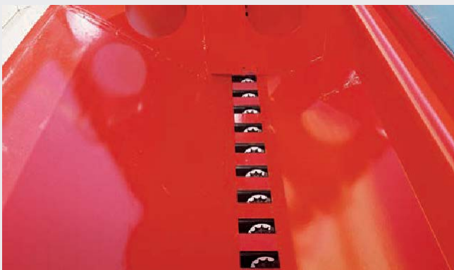
Feeding units under flat hopper's bottom eliminates changes to feeding amount in hilly conditions.
